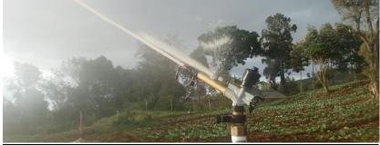
Highly efficient sprinkler rotating in full circle or part circle, impact type, operating at medium pressure (2-5 bars) with replaceable sprinkler nozzles and double hole water outlet, it ensures uniform water distribution. It can be used for irrigation of any kind of field crops and vegetables. It is appropriate for use with stationary and travelling systems. It may also be used for industrial applications for example, mines, construction sites and for dust.
